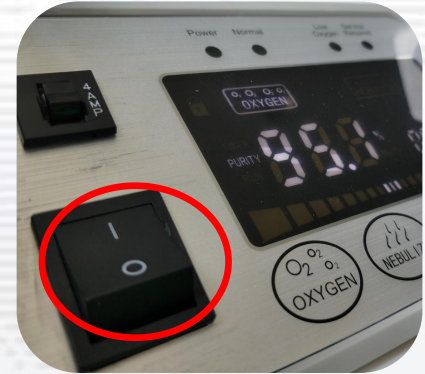
Turn on the Switch at "I" position to run the machine
