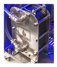
The large, 15 plate electrolysis cell and tank capacities in the Hydrogen Technologies machine allow for efficient gas production at low electrical demand and low operating temperature, allowing the generator to produce a full 1800+ liters of gas per liter of water used. The colder the machine can operate at, the higher the gas's quality and the generator's increased life span and its components.
